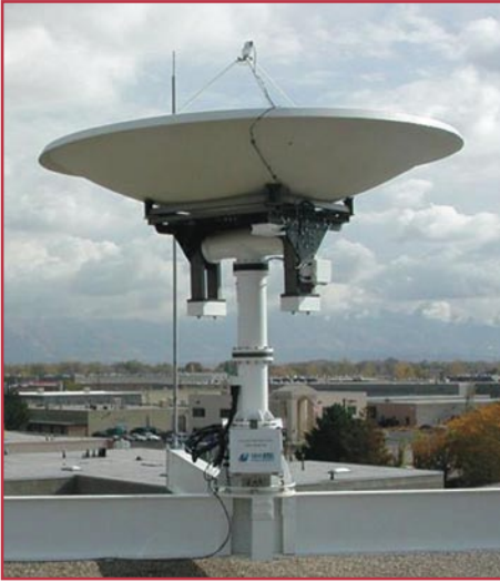
Figure 2—The Remote Sensing Applications Center's MODIS receiving station in Salt Lake City, UT, downloads imagery directly from the Terra and Aqua satellites six to eight times daily.
