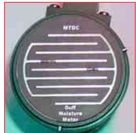
Figure 3—The bottom of the sample chamber is a printed circuitboard containing two interlocking finger sensor electrodes attached to a movable piston.
