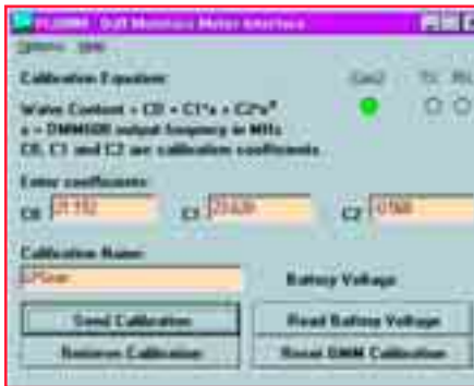
Figure 5—The PCDMM duff moisture meter interface software. A user-defined calibration curve, such as for gravimetric moisture content, can be added by setting the three calibration coefficients. The DMM600 display alternates between the standard volumetric moisture content and the user-defined calibration for each measurement.
