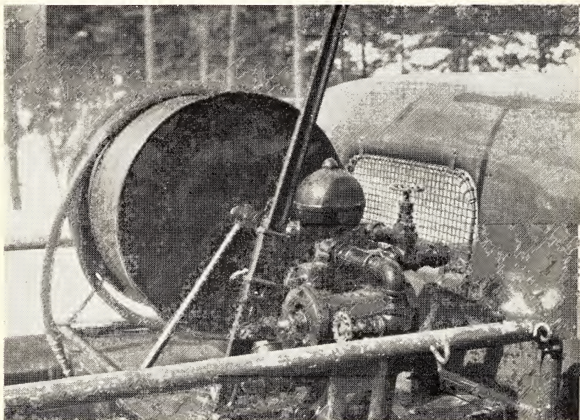
Portable hand-operated water pump constructed from a used threshing machine unit.
