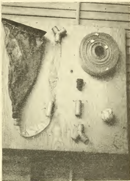
Fibrous water hose, gravity intake, and connections.
