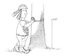
Figure TD-6. DBH Measurement. The diameter tape should carefully be pulled tight around the tree without twists or bends.
