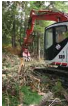
Figure 39. Mechanical slash reduction typically involves some type of attachment to an excavator, a bobcat, caterpillar, or similar machine.
