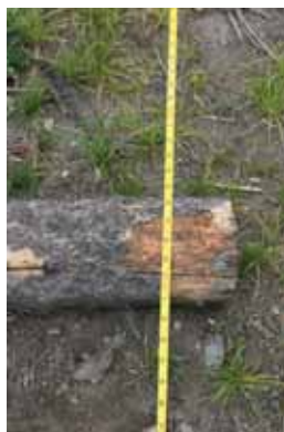
Figures 70. The tape must cross the whole log (left), not just a corner (right) to be counted in a transect.
