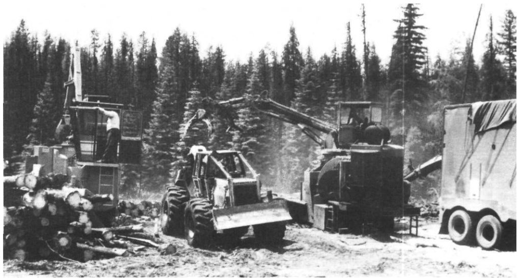
Figure 3.—Log trimmer (left), grapple skidder (center), and mobile chipper (right) at a landing site.
