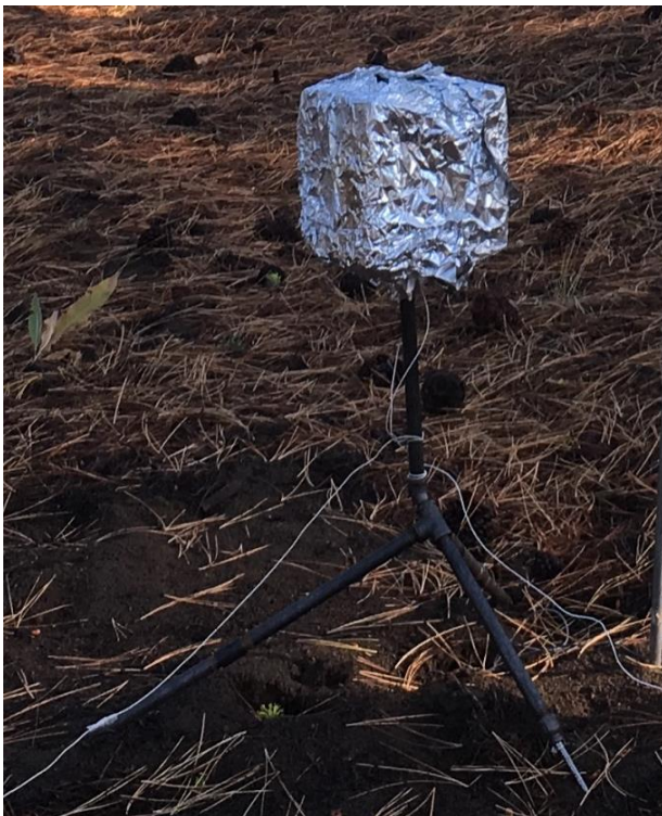
Figure 11. Camera on tripod with trigger wire.
