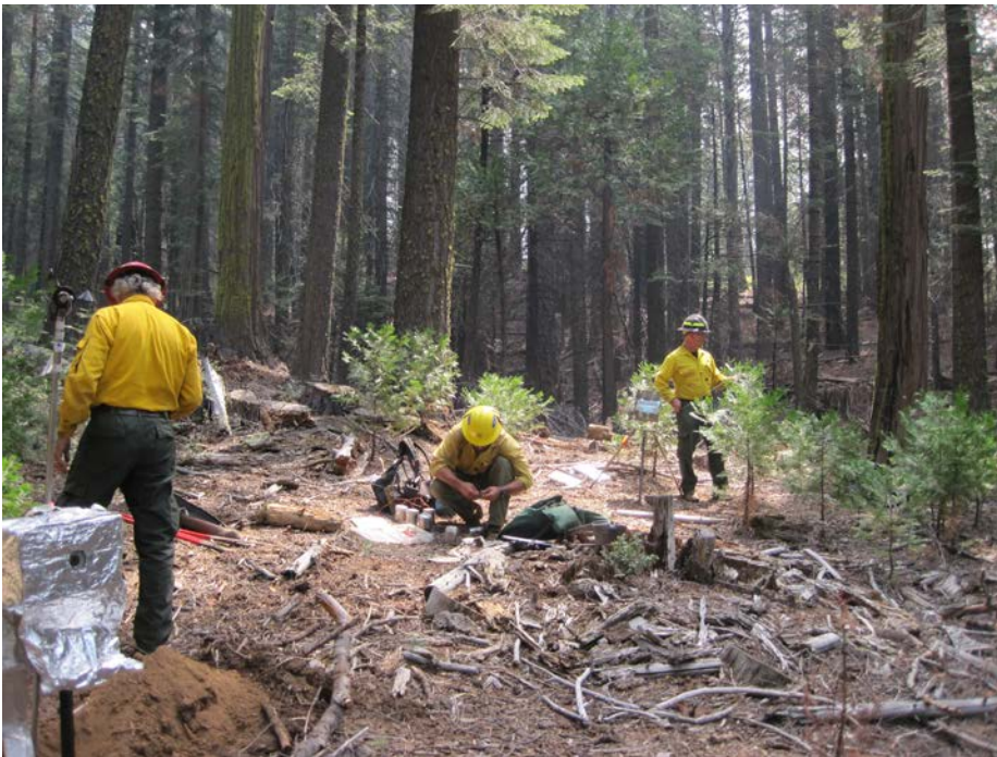
Figure 3: Examples of fire behavior equipment set up at the Willow Fire at plot 2. Viewing diagonally from left to right next to the workers are the heat flux sensor, the thermocouple cans (to be buried to measure spread rate), and in the distance is the video camera box.
