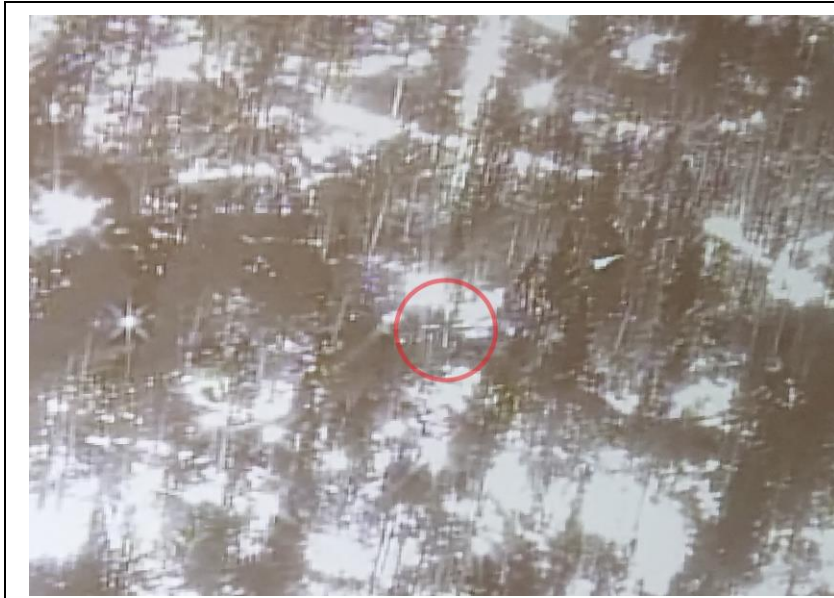
Figure 6. Infrared radiation from duff consumption imaged by a California Air National Guard drone on plot 8 at 19:29 PDT - about 2.5 hours after the flaming front spread through the plot. The crosshairs near the center of the image are close to plot center. Cool areas are dark while hot areas (e.g., duff and log consumption) are bright.
