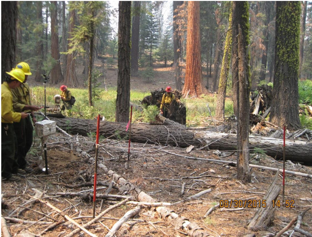
Figure 3: Examples of fire behavior equipment set up at the Rough Fire at plot 18, in the Boulder Creek giant sequoia grove. Equipment from left to right next to the workers are the heat flux sensor and anemometer, the video reference poles (to estimate flame lengths and spread rate), and in the distance is the video camera box.
