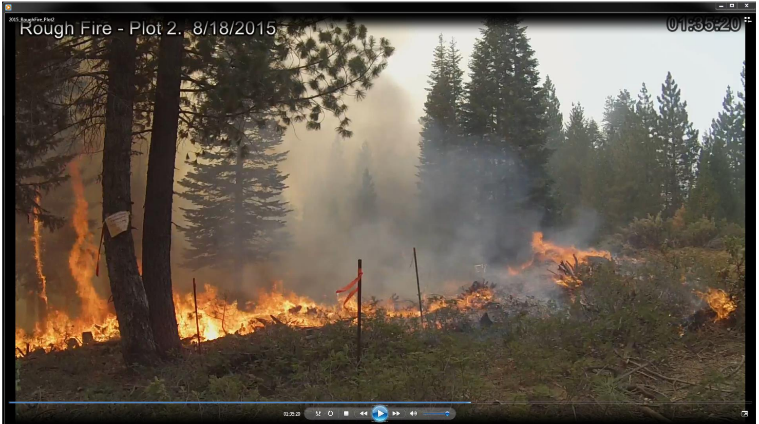
Figure 8. Plot 2 burning, photo captured from video. All three four-foot reference poles are visible in center of the photo, and the heat flux sensor in the background (just right of center). The day the site burned is captured on the video.
