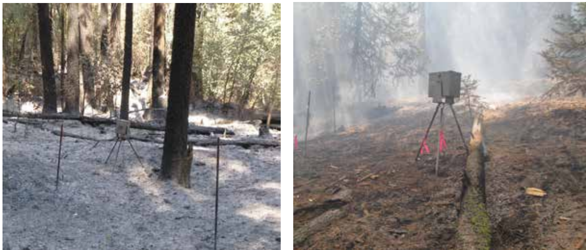
Figure 5: Example of fire resistant video camera box (center of image) at two Rockefeller Grove sites, post-fire.
