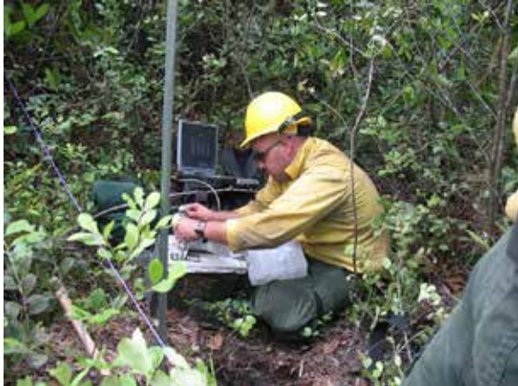
Figure 2. Installing fire behavior sensors at one of sites.
