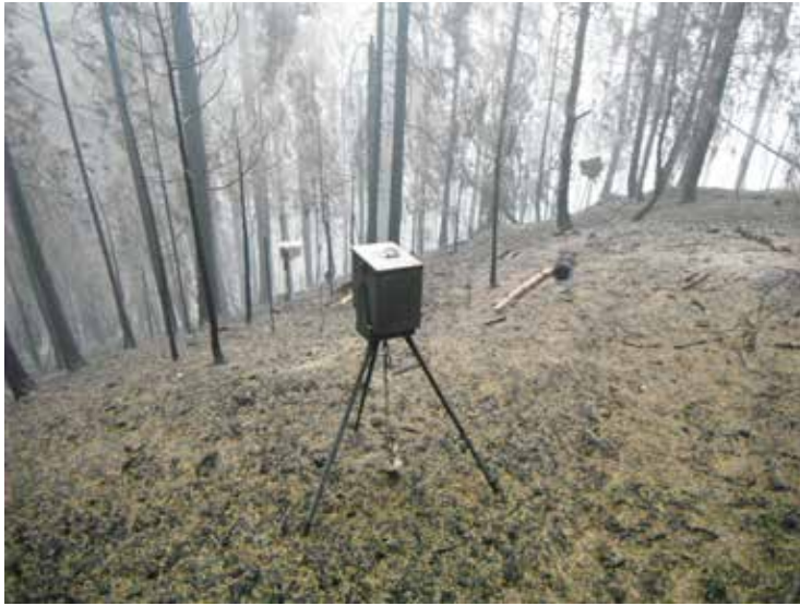
Figure 4: Examples of fire behavior equipment set up at the Beaver Fire. Upper photo shows camera box in foreground, lower photo shows heat flux sensor and anemometer.
