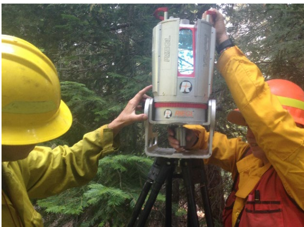
Figure 3. Crew members setting up the TLS scanner at a plot on the Ferguson Fire.
