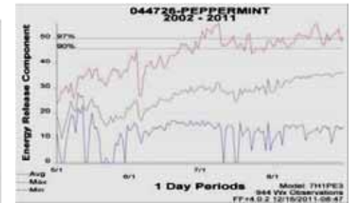
Figure 41. Lion Fire Interactions - Energy Release Component (ERC) at the Peppermint RAWS during May through August, for 10 years 2002 to 2011 using fuel model H shows average ranging from about 10 to 36 with extremes from 0 to 58.
