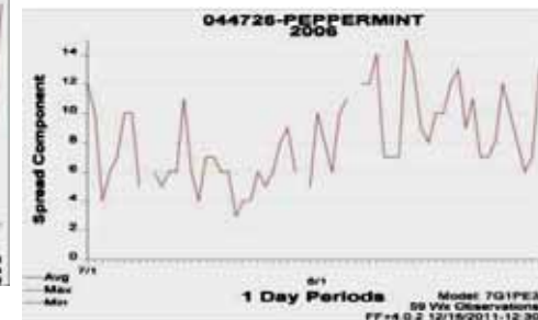
Figure 77. Maggie and Tamarack Fires - Spread Component at the Peppermint RAWS for July and August, 2006 shows a range from 3 to 15 feet per minute. (Fuel Model G).
