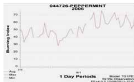
Figure 33. Maggie and Tamarack Fires - Burning Index at the Peppermint RAWS during July and August, 2006, ranged from about 30 to 75. The model’s configuration predicted flame lengths would have ranged from about 3 to 7.5 feet. The BI for the period generally was at about average during June above average during August.
