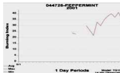
Figure 34. White Fire - Burning Index at the Peppermint RAWS during May, 2001, ranged from about 25 to 45. The model’s configuration predicted flame lengths would have ranged from about 3.5 to 4.5 feet. The BI for the period about average.
