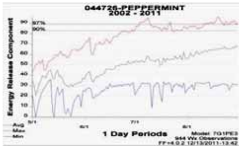
Figure 36. Energy Release Component (ERC) at the Peppermint RAWS during May through August, for 10 years 2002 to 2011 using fuel model G shows average ranging from about 20 to 68 with extremes from 10 to 95.
