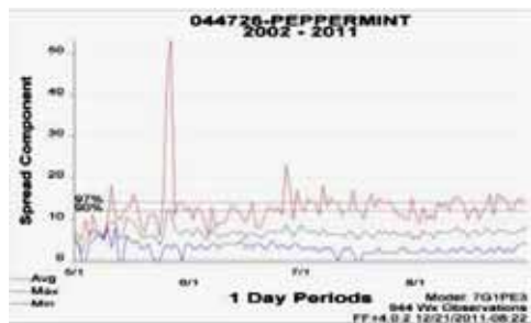
Figure 74. Spread Component at the Peppermint RAWS during May through August for 10 years 2002 to 2011 showing average ranges from about 2 to 12. (Fuel Model G). The high number (50+) is either an outlier buried in the data set or very windy few days.
