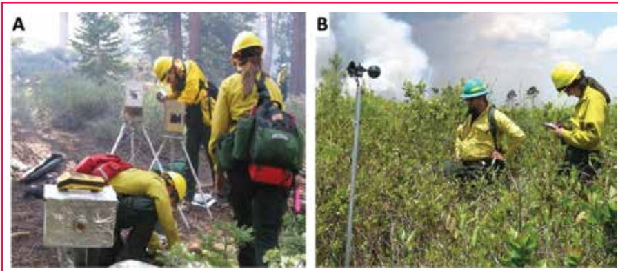
(A) Members of the Fire Behavior Assessment Team setting up the fire-resistant video cameras and radiant heat flux sensor on the Crag Fire in 2005 (photo: Rosalind Wu, Forest Service) and (B) gathering fuels data near the anemometer on the Georgia Bay Complex in 2007 (photo courtesy of Adaptive Management Services Enterprise Team).
