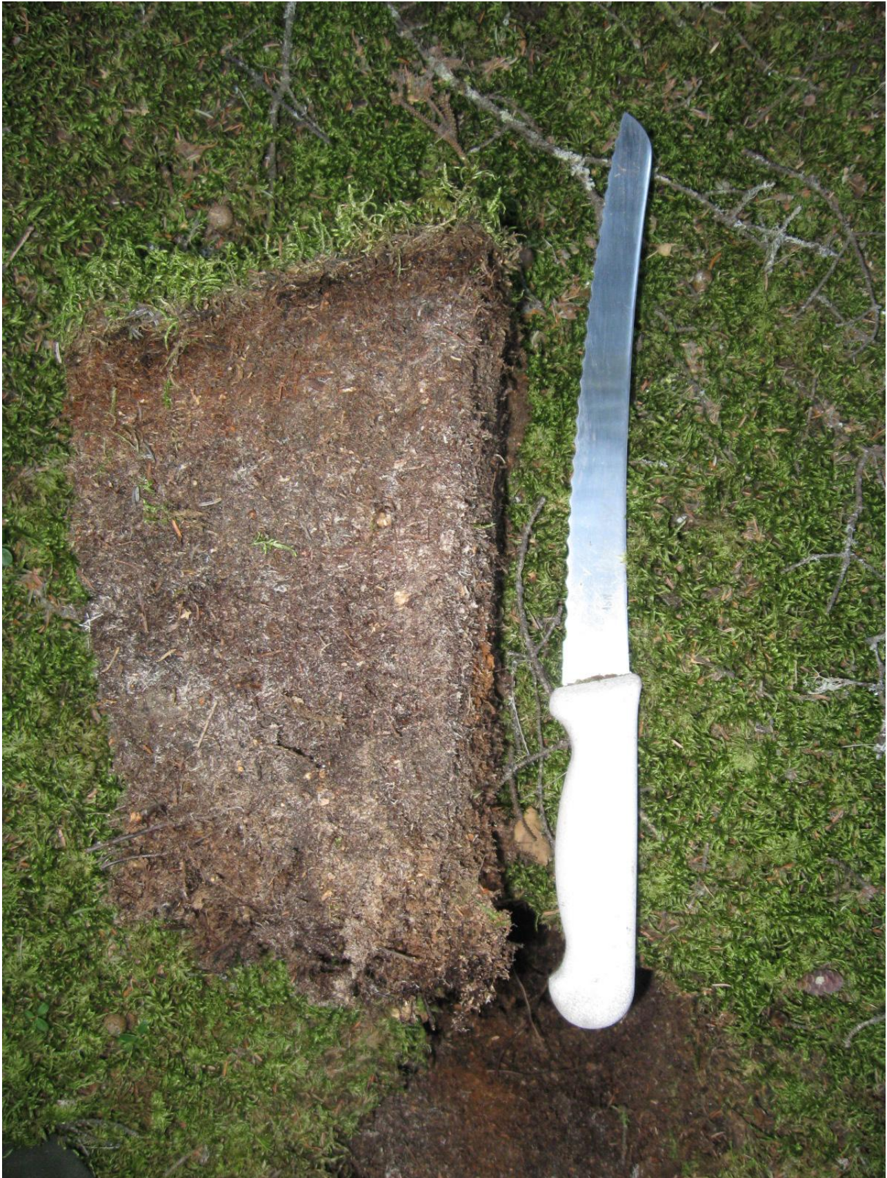
Figure 7. Duff plug showing the live moss, dead moss, and upper duff layers. The steel blade on the bread knife is 9-3/4" (25 cm).
