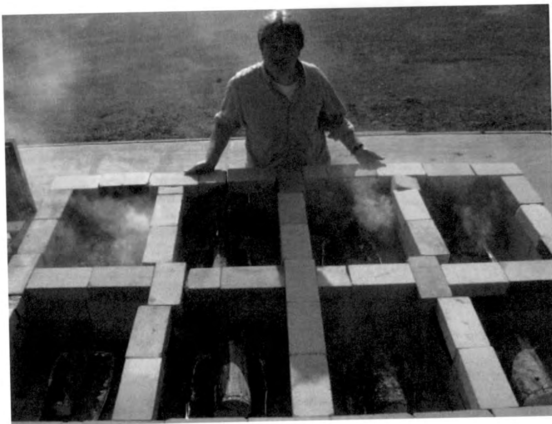
Figure 7. Partitioned table on which CWD samples were allowed to smolder. Brick cells sheltered the samples from wind and heat from adjacent samples.
