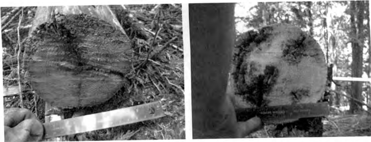
Figure 13. Samples numbered 51 (left) and 126 (right). Here we see these are predominantly sound wood with the exception of some channels of interior decay. In both cases this interior decay became an ignition point from which smoldering in the sound sections was initiated. The pictured ruler is 15cm for scale.
