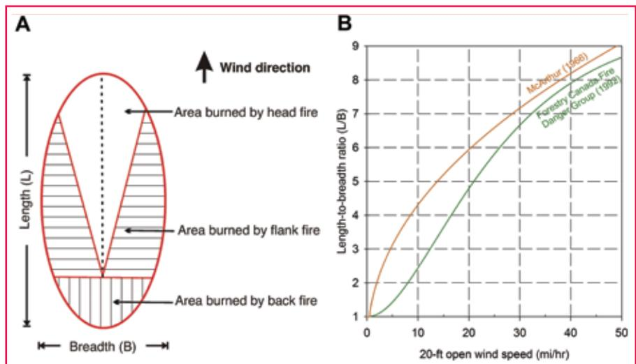
**Figure 1.** —(A) Schematic diagram of a simple elliptical fire growth model (after Van Wagner 1969) with the point of ignition represented by the junction of the four area growth zones and (B) the length-to-breadth ratio of elliptical shaped surface and crown fires in conifer forests on level to gently undulating terrain as a function of wind speed for conifer forests (Forestry Canada Fire Danger Group 1992) and grasslands (McArthur 1966).
