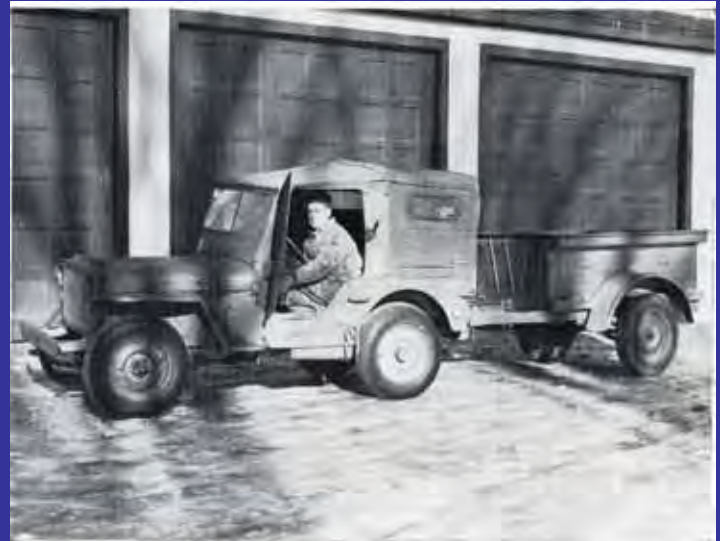
JEEP AND TRAILER CARRYING PUMP UNIT AND HOSE AVAILABLE FOR USE IN DIFFICULT LOCATIONS
