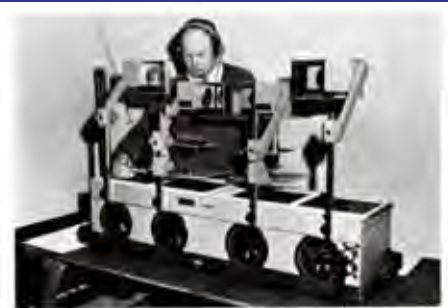
Forest fire suppression training. With the forest fire simulator trainees are subjected to the pressures and problems encountered on an actual fire. The four overhead projectors superimpose increasing size of perimeter, smoke and fire movement on the landscape.
