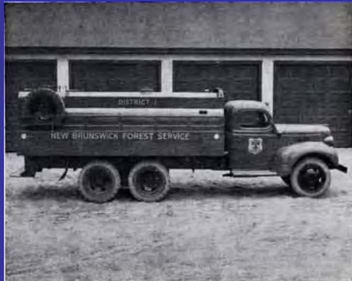
Tanker with Tandem drive rear axles. These are more satisfactory to woods roads than single rear axles on the dual wheels.
