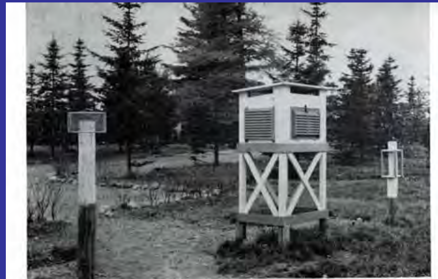
METEOROLOGICAL EQUIPMENT AT THE ACADIA FOREST EXPERIMENT STATION. The apparatus shown is quite typical of the twenty-one forest weather stations now established in New Brunswick. The ventilated box in the centre contains instruments for measuring the temperature and relative humidity of the air. Mounted on the posts to the left and right of the picture are an evaporimeter and a rain-gauge respectively.
