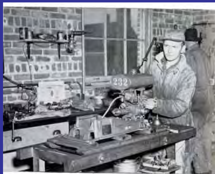
OVERHAULING PUMP UNITS AT FREDERICTON SHOP IN WINTER IS PART OF ROUTINE MAINTENANCE PROGRAM
