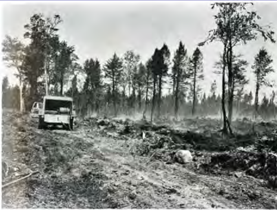
ONE OF THE DEPARTMENT'S 52 TANKERS AT WORK EACH TANKER HAS A CAPACITY OF 800 TO 1000 GALLONS
