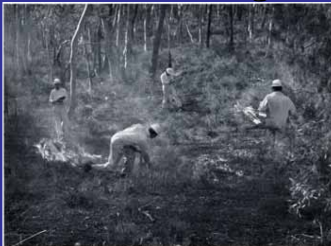
Experimental fire behaviour studies in dry sclerophyll Eucalypt forest; Black Mountain, A.C.T. These are low intensity fires burnt during late autumn. Metal markers are used to locate the perimeter at two minute intervals.
