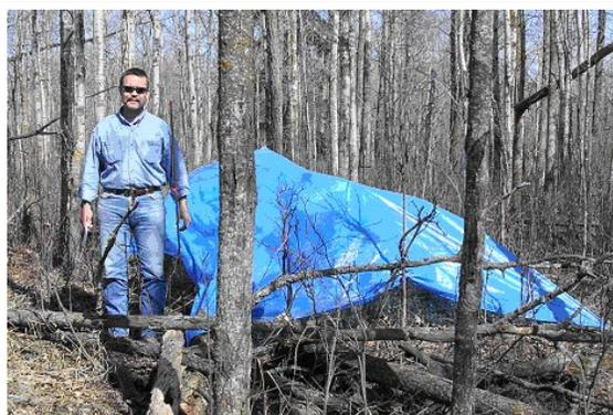
Steve Otway at one of his plastic fuel moisture "exclusion tents" designed to artificially decrease long-term fuel moisture levels in the deeper layers of aspen forest floor by excluding rainfall in order to extend the range in the DMC and DC components of the Canadian Forest Fire Weather Index System.
