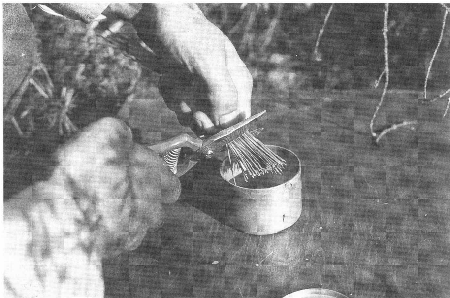
Figure 3.18. Fuel samples are clipped into a can, weighed, dried, and weighed again to determine moisture content. Photo by Melanie Miller. From Norum and Miller (1984).
