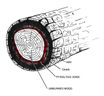
Thus, if we examine a cross section of a partially burned piece of wood we see from the surface inward first a thin layer of ash, next a layer of char, then a layer, usually shading from dark to light brown, where the pyrolysis has been taking place, and finally unburned wood. The speed with which the pyrolysis layer moves through the wood determines its burning rate.
