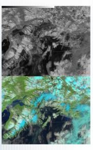
The imagery at left centered over Prince William Sound is from the Suomi NPP VIIRS instrument at 2156Z on July 10, 2015. The top image is the 1.61 µm snow/ice channel alone. The bottom image is the Natural Color RGB which assigns the 1.61 µm snow/ice channel to the red component, the 0.84 µm channel to the green component, and the 0.64 µm channel to the blue component.
